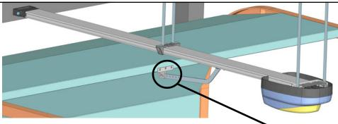
Hang the arm to the bracket and fix it with the nut and bolt TE 8x25
