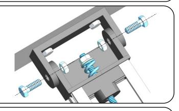
Bend the brackets according to the measure **A**. This measure is obtained leveling the guide with the ceiling
