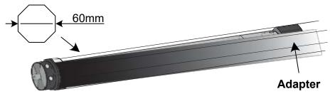
First of all make sure that the tube is octagonal and 60mm diameter.
