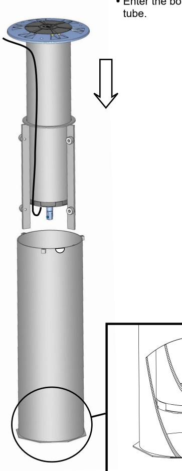
• Enter the bollard letting the wheels in the tube.
