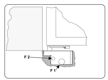
Note: while positioning the box, keep in mind the minimum distance there must be between the pillar and the centre of rotation of the gate hinge.
