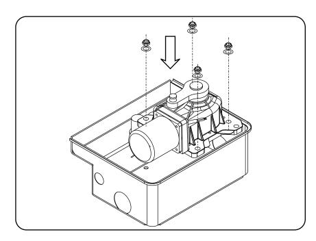
Insert the ball in the pin located on the box and fit the gate anchorage lever (L1)
